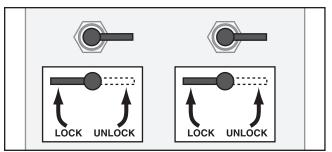
Figure 3. Configuration to freely slide table.
